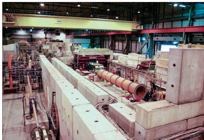
A photograph of the experimental area of NA63, seen in the right half of the figure, at the North Area at CERN. The long orange tube is a helium vessel through which the beams of hundred giga-electron-volt electrons and photons pass from the target to the detectors. (Image credit: Mikkel D Lund/NA63.)
